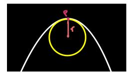
The curvature at point p is the inverse radius of the circle which touches p, i.e.  $k = \frac{1}{\pi}$ .
